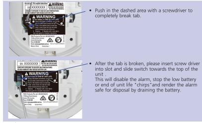
A WARNING! Failure to discharge alarm as instructed prior to disposal may create potential for lithium battery related fire or hazard.
